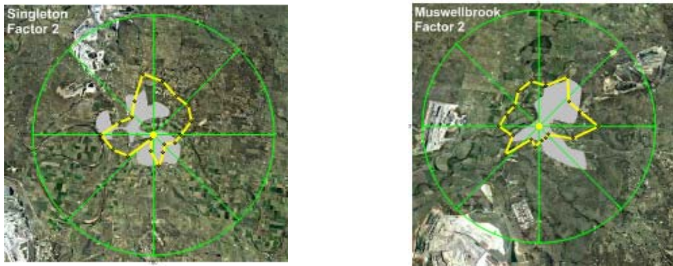
Figure 27 CPF plot of Factor 2 (Vehicle/Industry) at Singleton (left) and Muswellbrook (right). The highest Vehicle/Industry contributions at Singleton (left) were associated with winds from the north and west i.e. in the direction of the coal mines and most sectors at Muswellbrook (right) but there are contributions from most other wind directions indicating local sources.
