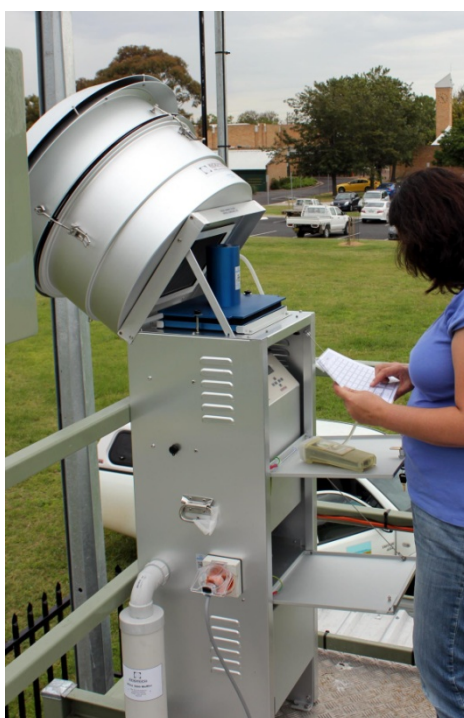
Figure 7 CSIRO high volume sampler at Singleton with flow rate calibration being carried out
