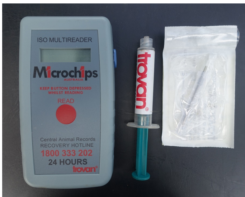
Figure 10 Microchip scanner, implanter and needle with microchip
