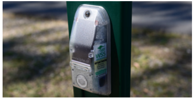
Figure 6 Virtual fence post with sensor on the side of a road. Approaching car headlights activate the sensor which emits sound and light to deter animals from crossing the road. (Wildlife Safety Solutions)
