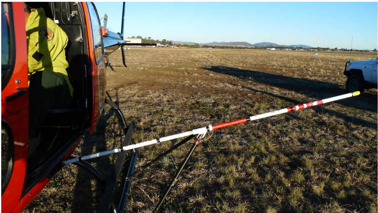
Fig. 4 Distance boom mounted on the left-hand side of the Eurocopter AS350 Écureuil helicopter used in the survey. The distance bins used in the surveys (0-20 m, 20-40 m, 40-70 m, 70-100 m and 100-150 m) are indicated by the black bands on the boom.
