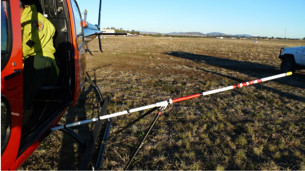
Fig. 5 Distance boom mounted on the left-hand side of the Eurocopter AS350 Écureuil helicopter used in the survey. The distance bins used in the surveys (0-20 m, 20-40 m, 40-70 m, 70-100 m and 100-150 m) are indicated by the black bands on the boom.
