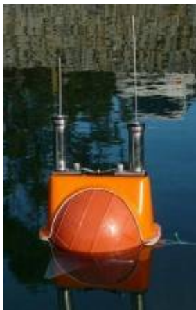
Figure 91 Satellite and VHF PTTs on buoy. Photo: Eric King, Australian Antarctic Division.
