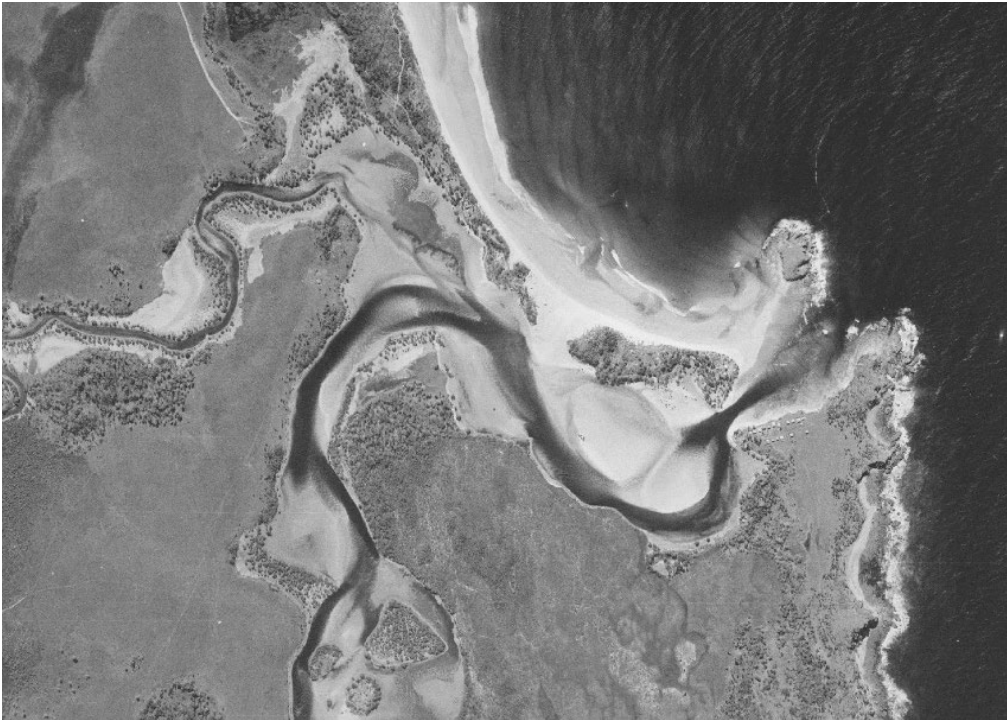
Figure B.2 1958 – showing potential wave overwash at one location and substantial sand accretion along Sandon Beach and within Sandon River
