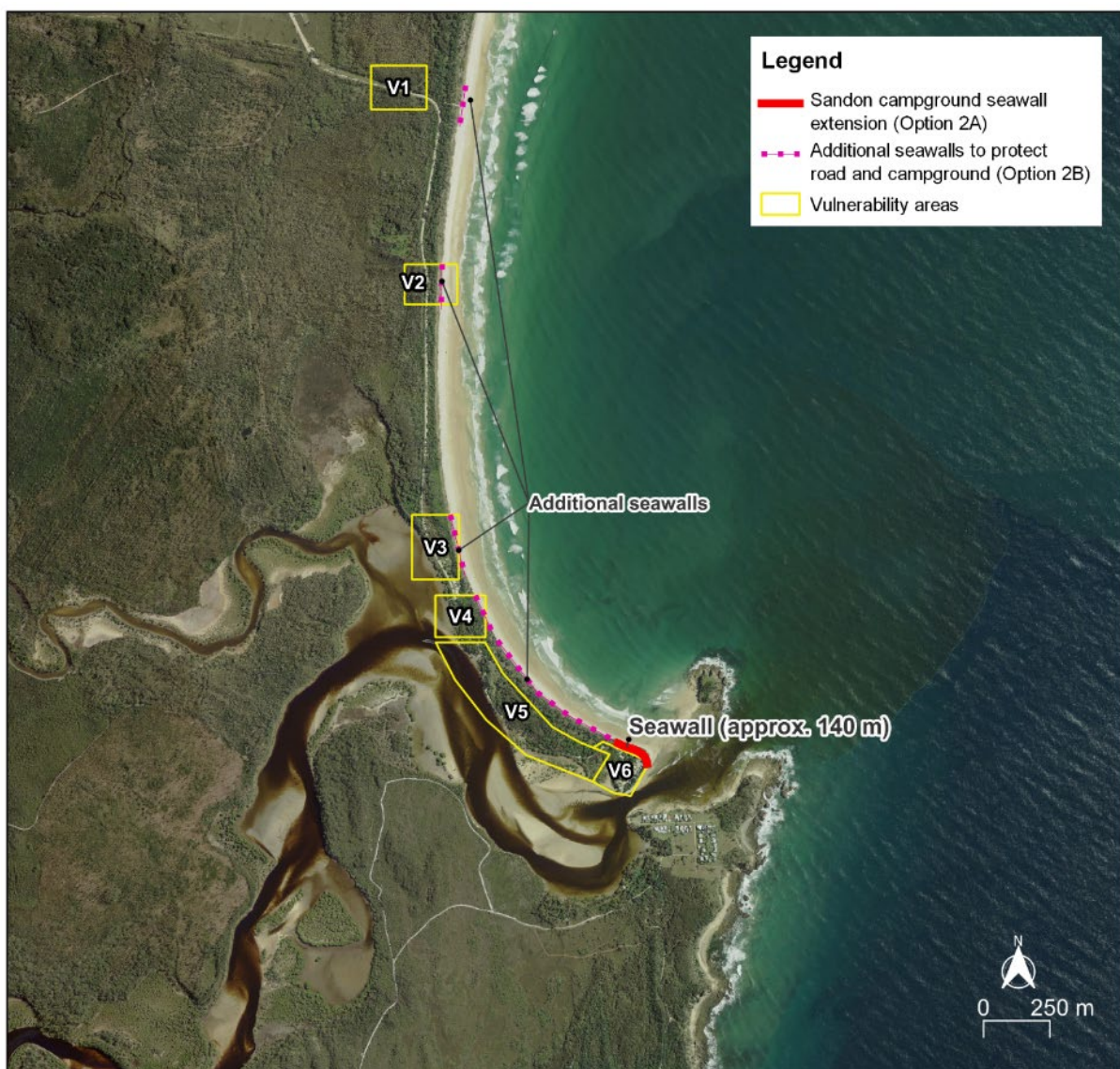
Figure 10 Aerial view of locations for proposed seawall to protect Sandon River campground (option 2A) and the campground and access road (option 2B)
