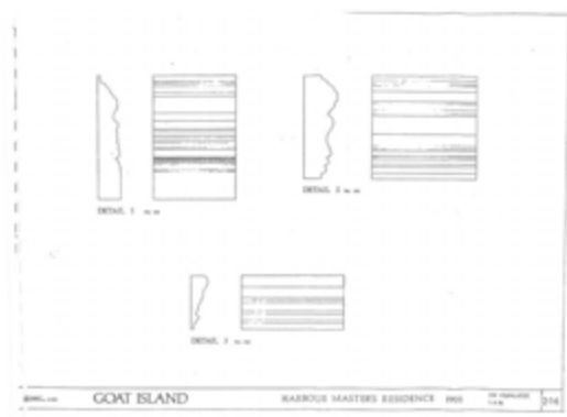
Joinery details (from Appendix A, Beebe Ed et al, June 1997 The Harbour Master's Residence, Goat Island, Sydney Harbour National Park: A Conservation Plan )
