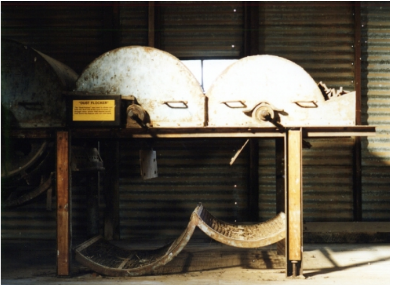
Figure 14 The dust flocker in the Kincheha woolshed. This machine was used to extract sand particles from the wool. PF 2001 photograph
