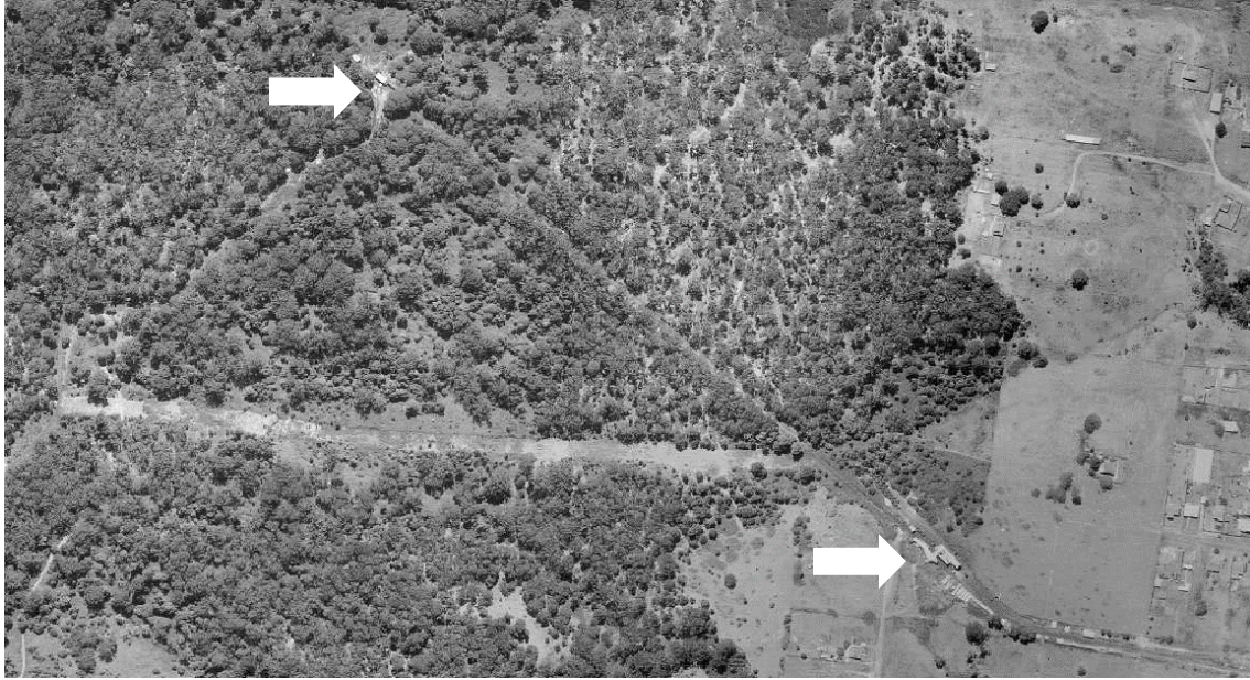
Plate 2: 1948-51 historical aerial imagery showing the 'old' incline route with the top (west) and lower (east) ends indicated. This incline was located to the northeast of the pit top, note the powerline easement located south of this system (source: WCC public imagery; Department of Customer Service 2020).
