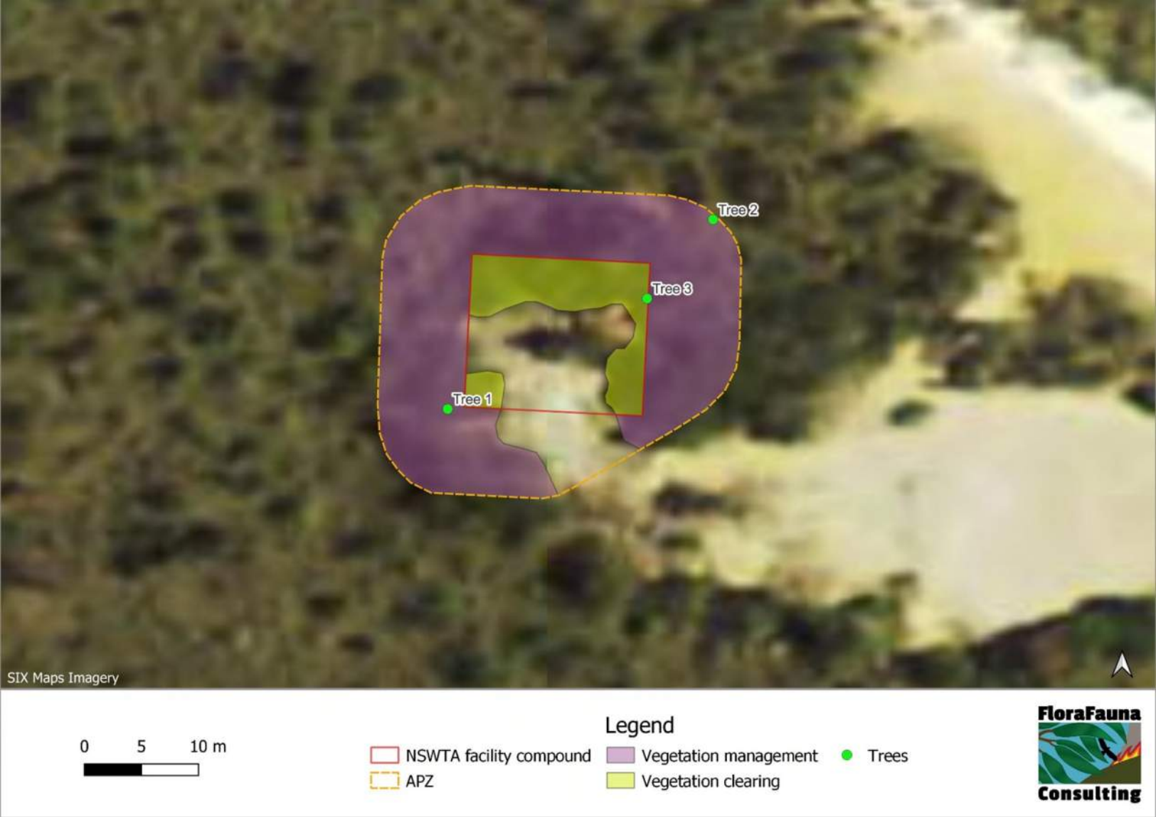
Figure 22: Relative position of the proposed NSWTA compound and APZ, and extent of associated vegetation clearing and management
