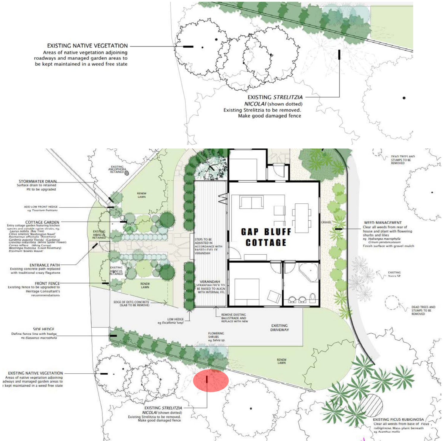
Figure 9. Landscape plan of Gap Bluff Cottage showing location of Strelitzia Nicolai for removal (Source: Trish Dobson Landscape Architecture. Please see submitted landscape Drawings for more detail.)
