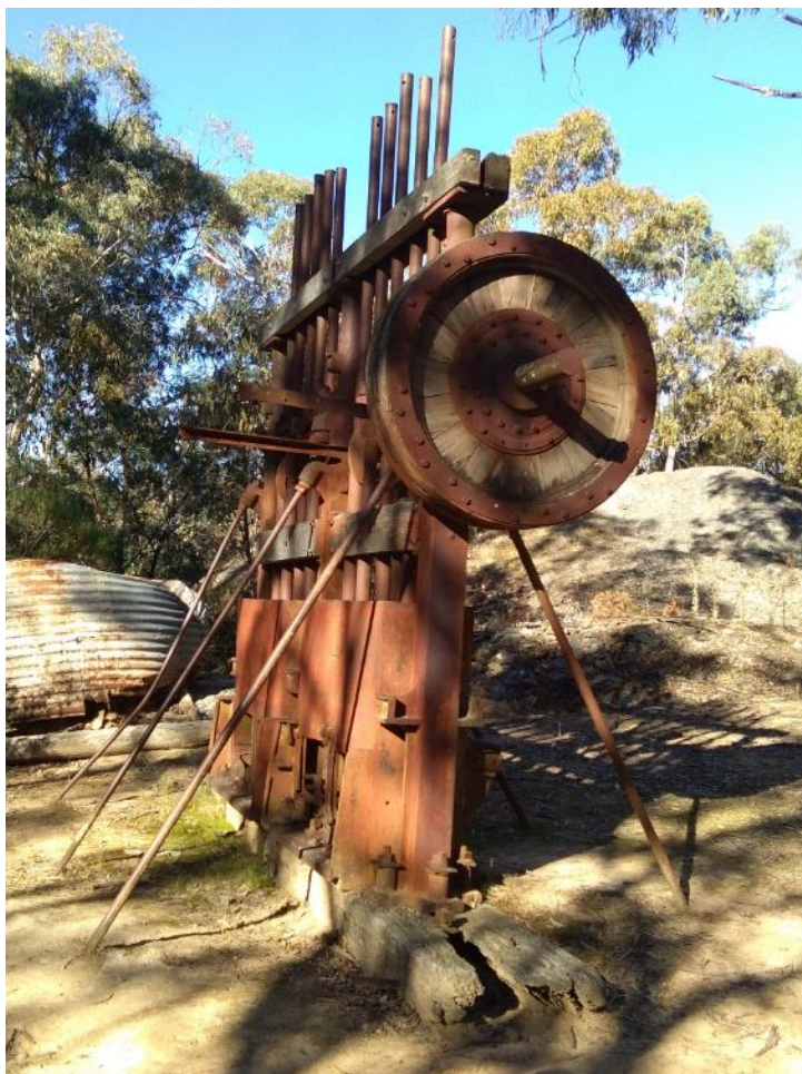
Photo 16 Stamper battery, Valentines Mine. M Billington/DPE
