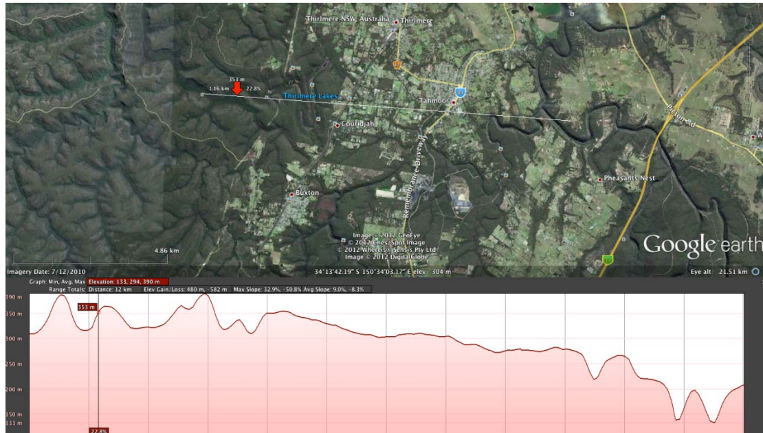
Figure 3-6. Cross section drawn from Google Earth showing Thirlmere Lakes topographically above much of the land surface to the east (copyright; Google Earth; 2012 ©Whereis@Sensis Pty Ltd; Image©2012GeoEye).
