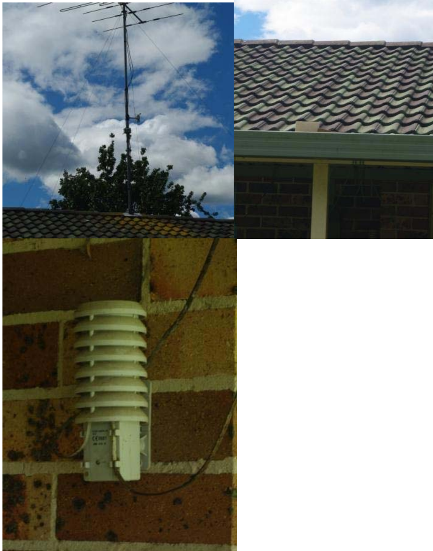
Figure 4-2. Elements of the Thirlmere Lakes Automatic Weather Station. From top left, clockwise, anemometer, tipping bucket rain gauge, and temperature and pressure probe housing.
