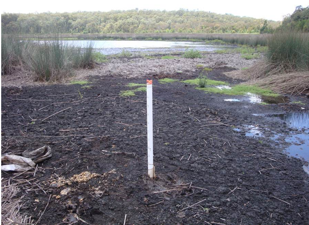
Figure 5-31. Lake Gandangarra piezometer at installation, 10 February 2012.
